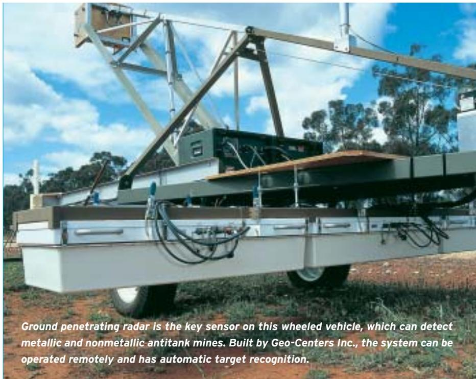
Ground penetrating radar is the key sensor on this wheeled vehicle, which can detect metallic and nonmetallic antitank mines. Built by Geo-Centers Inc., the system can be operated remotely and has automatic target recognition.
